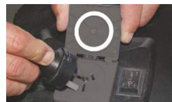
■ Sander power point and on/off switches
