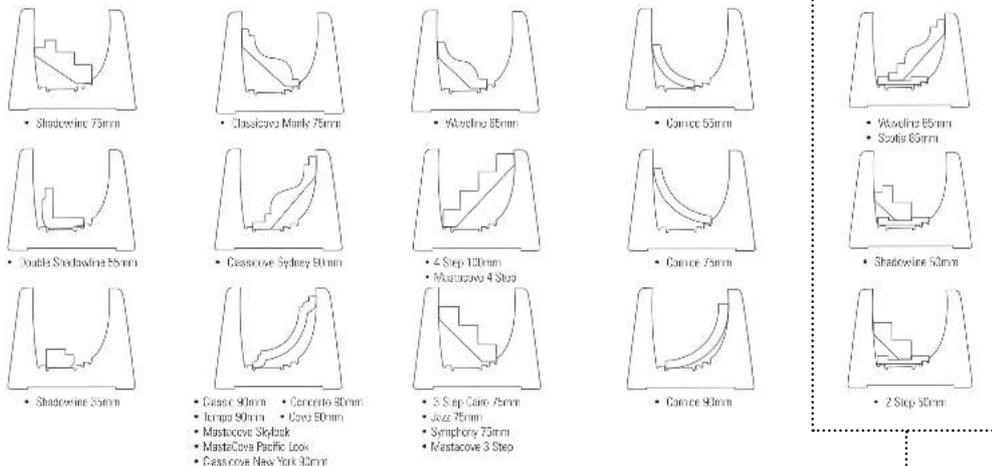
The plastic mitre box is able to accommodate twelve different profiles of cornice. Three further cutting profiles are achieved with addition of the 14-410 timber insert.
