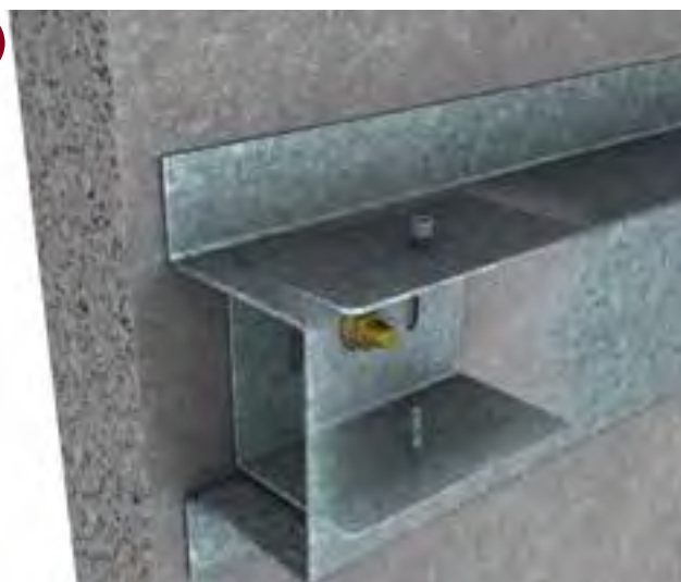
■ TOP HAT FIXED TO CONCRETE ANCHOR SIZE TO CONCRETE/MASONRY 8-10mm AS SPECIFIED. TOP HAT TO CLEAT WITH #12 TEK SCREWS AS SHOWN
