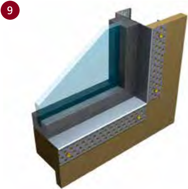
■ REVEAL BEAD INSTALLATION
