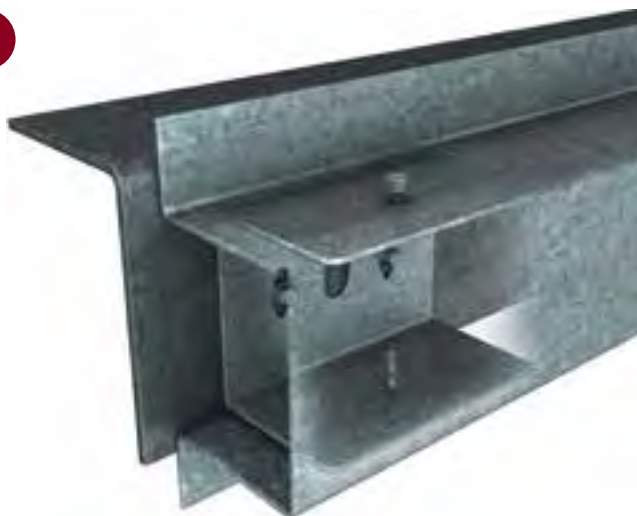
■ TOP HAT FIXED TO STEELWORK FIXINGS: CLEAT TO STEELWORK AND TOP HAT TO CLEAT WITH #12 TEK SCREWS AS SHOWN
